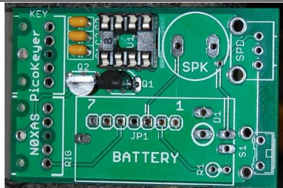
Find the speaker and install it in the location marked SPKR. The speaker may be marked with a + on one side; don't worry about polarity as it can be installed either way. Make sure the speaker is inserted fully into the holes before soldering. Don't bend the leads of the speaker; you may want to use a bit of adhesive tape to hold it in place. Don't spend too much time soldering the speaker or it may be damaged.
